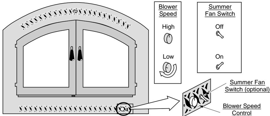
**Note:** The blower will shut off when the doors are opened.
