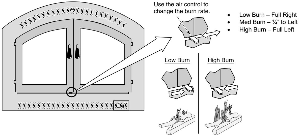
**Warning:** The air control becomes hot during operation - use gloves or a tool to prevent burns.
