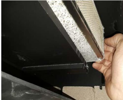
3. Install new combustor making sure that the side insulation and the combustor top and bottom gasket are in place.
